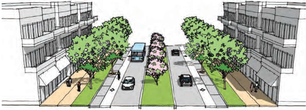
Figure 11 3-Lane Avenue w/ Parking Cross-Section
